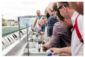
The rig allows researchers to see how a roof drainage system would stand up to any kind of stormwater event – from a shower through to a serious storm event. The pumping system is one of a kind and fully programmable, allowing it to model any possible storm event.
